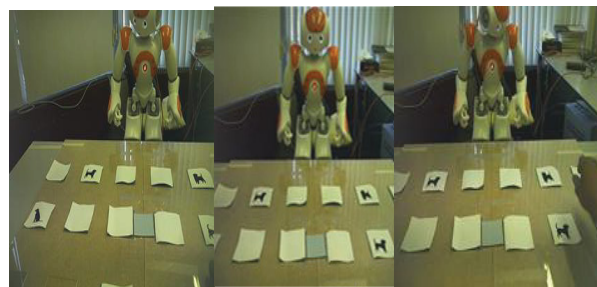
Fig. 1 Sequence of gaze cues for NAO tutor robot in "Help" condition. The NAO tutor looks at the card picked by the child, moves its head to the face of the child, and then to the matching card.
